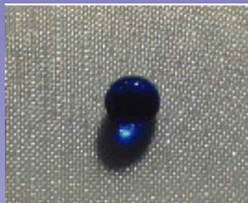
Hydrophobic through Plasma treatment: Surface rejects dirt and moisture
